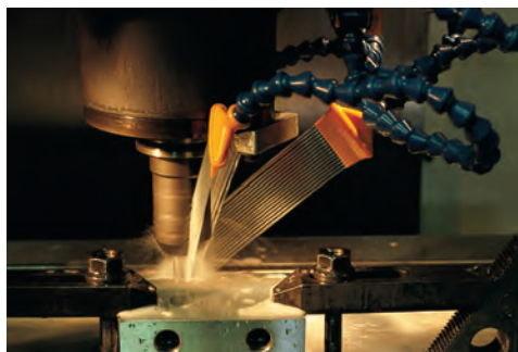
Flat nozzle with joint 16 hole Ø1.5
