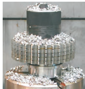
Clamp nut clamping sprockets during milling
